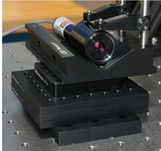
Figure 8 Source Laser with Beam Expander
