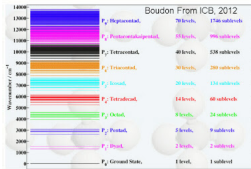
Figure 11. The four fundamental vibration frequencies of methane (three being degenerate oscillators with \nu_1 = \nu_3 = 2\nu_2 = 2\nu_4 ) form a vibrational structure with vibration levels grouped into polyads
