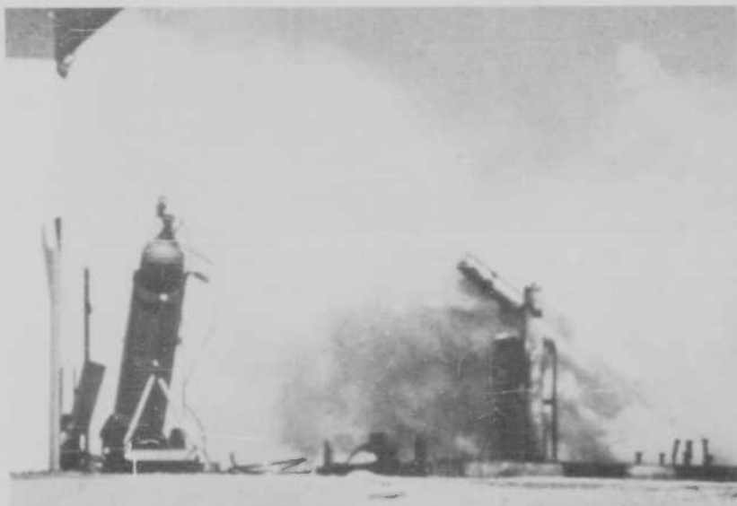
FIG. 2. A Static Ground Test of the Cyclops Unit Shows the Heavy Iodide Output as Demonstrated by the Color of the Smoke.
