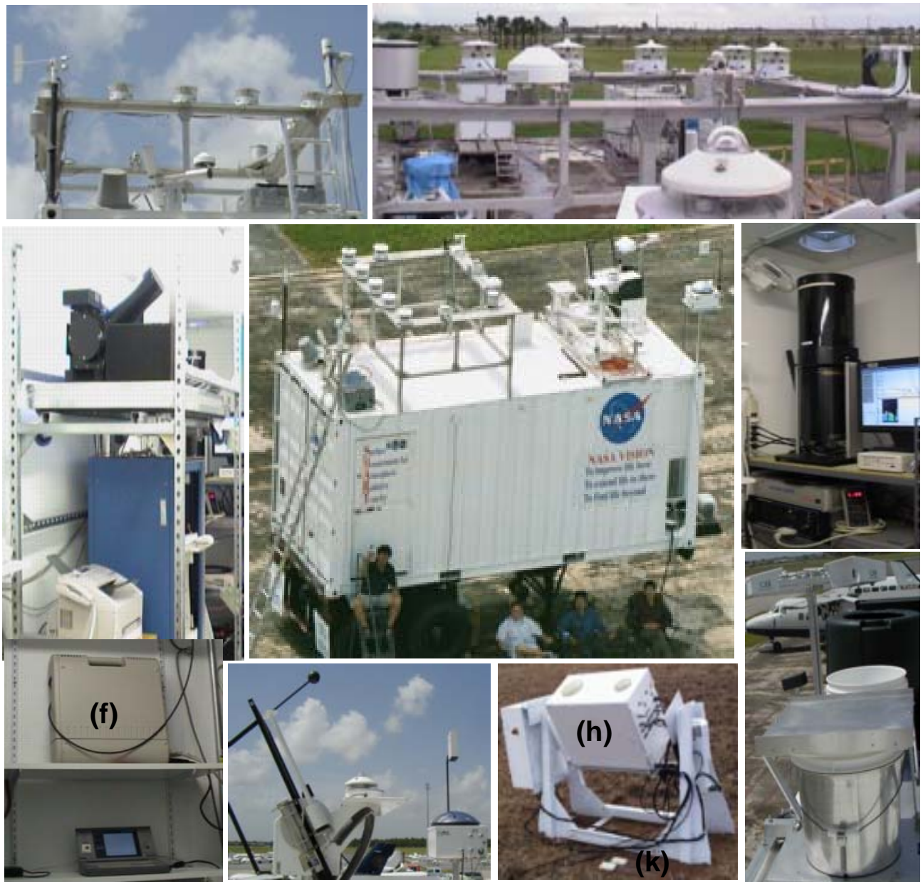
Figure G. 1. The latest version of the SMART system shown in center panel: (a 1 ) an array of broadband-total radiometers in ultraviolet, shortwave and longwave regions, (a 2 ) broadband-direct radiometers, (a 3 ) broadband-diffuse radiometers, (b) shadow-band radiometer, (c 1-2 ) sun photometers, (d) meteorological probes for atmospheric pressure, temperature, humidity, wind speed/direction, (e) interferometer, (f) solar spectrometer, (g) whole-sky imager, (h) scanning microwave radiometer, (k) soil moisture probes, (m 1 ) physical rain gauge, (m 2 ) optical rain gauge, and (n) micro-pulse lidar.
